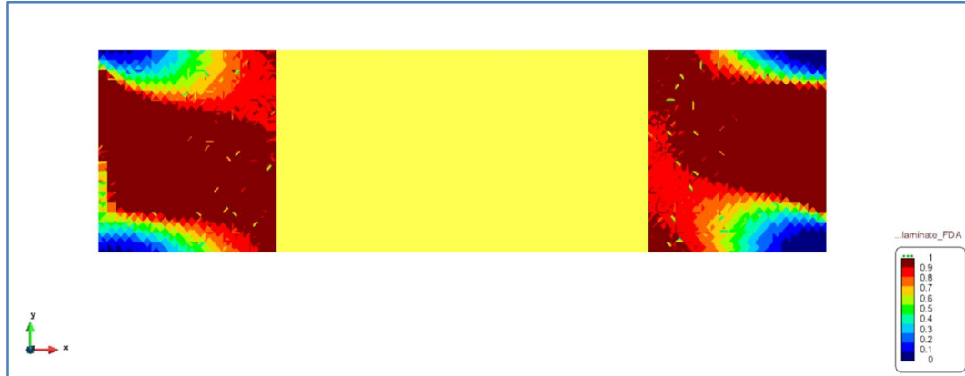
Figure 11: Damage state after 26311 cycles (24MPa).
