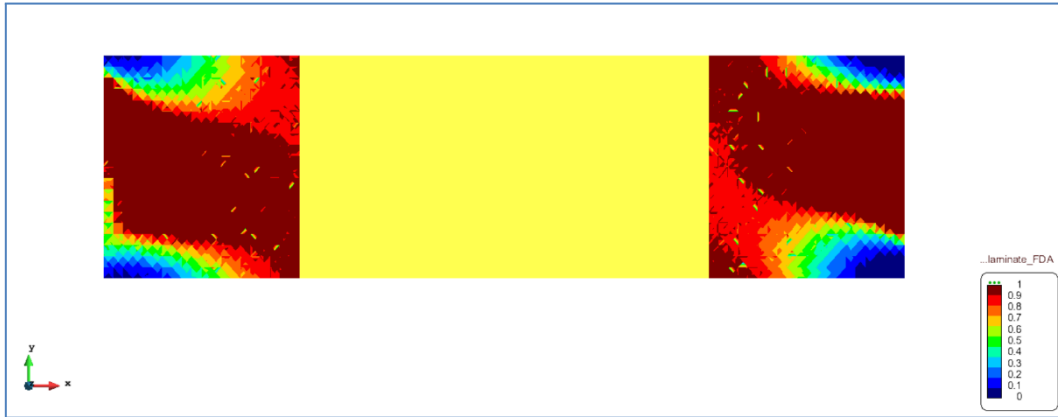
Figure 11: Damage state after 26311 cycles (24MPa).
