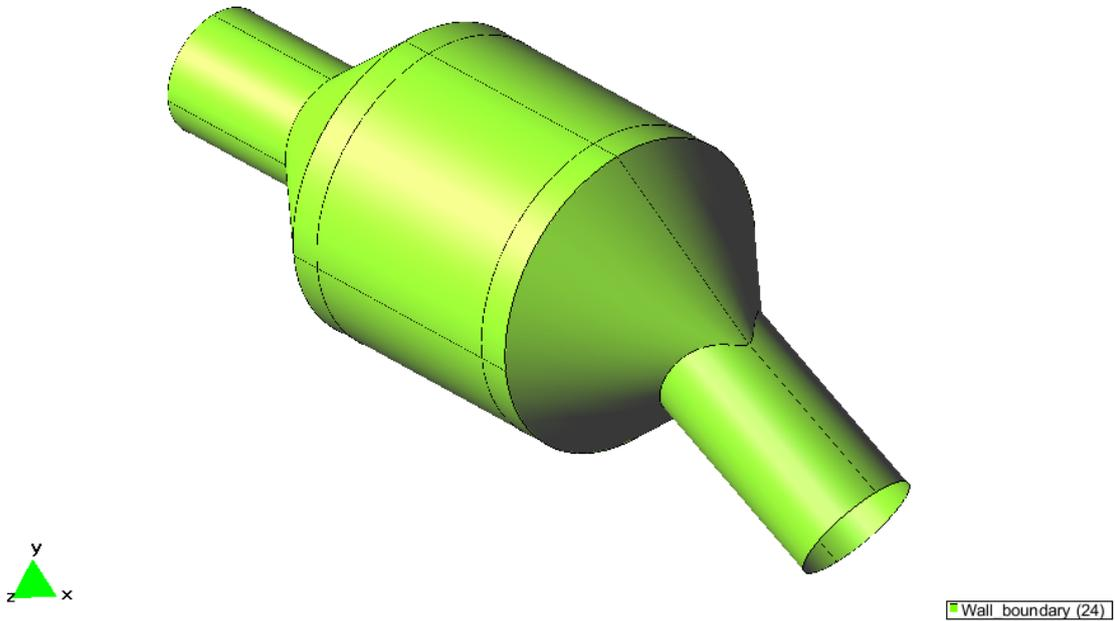
A **Fix Velocity** condition is further applied to the inlet surface of the model (in blue in the figure below) so that the velocity vector is fixed there to the value  $\mathbf{v} = (22.6, 0.0, 0.0)$  m/s. Finally, a **Pressure Field** condition is used to fix the the dynamic pressure to zero at the outlet surface of the control volume (in red in the figure below).
