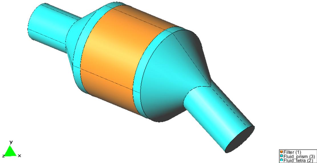
The Darcy's law matrix used to model the porous media is taken to be diagonal but anisotropic. The corresponding values of the viscous (D) and inertial (C) resistance terms are those in the table below. Note that the components of the Darcy's matrix are given with respect to the global axis system (X, Y, Z) so that the geometry must be conveniently oriented.
